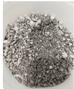
Figure 2: Cupola furnace slag to substitute the cement content in briquettes
